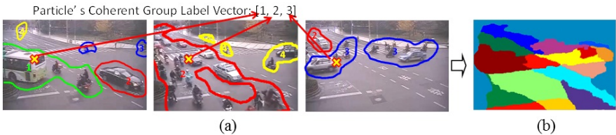
Figure 5. (a) Step 1: Coherent regions in the three TEFs have been assigned different cluster labels by Step 1 and are displayed in different colors); (b) Find semantic regions by clustering the cluster label vectors of the particles (best viewed in color).
